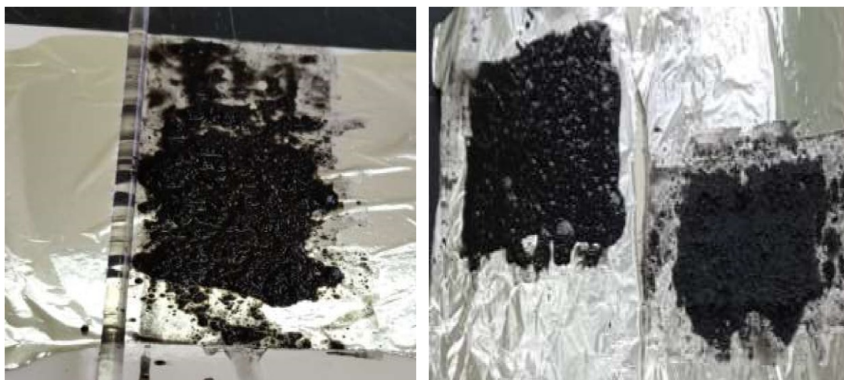
Figure 3. Mixtures coating on aluminium foil using glass rod
