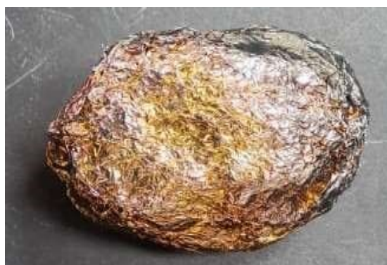
Figure 2. PKS wrapped by aluminium foil after physical steam in furnace
