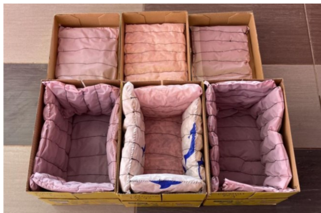
Figure 2.2 Attachment of the insulating materials onto the walls surface
