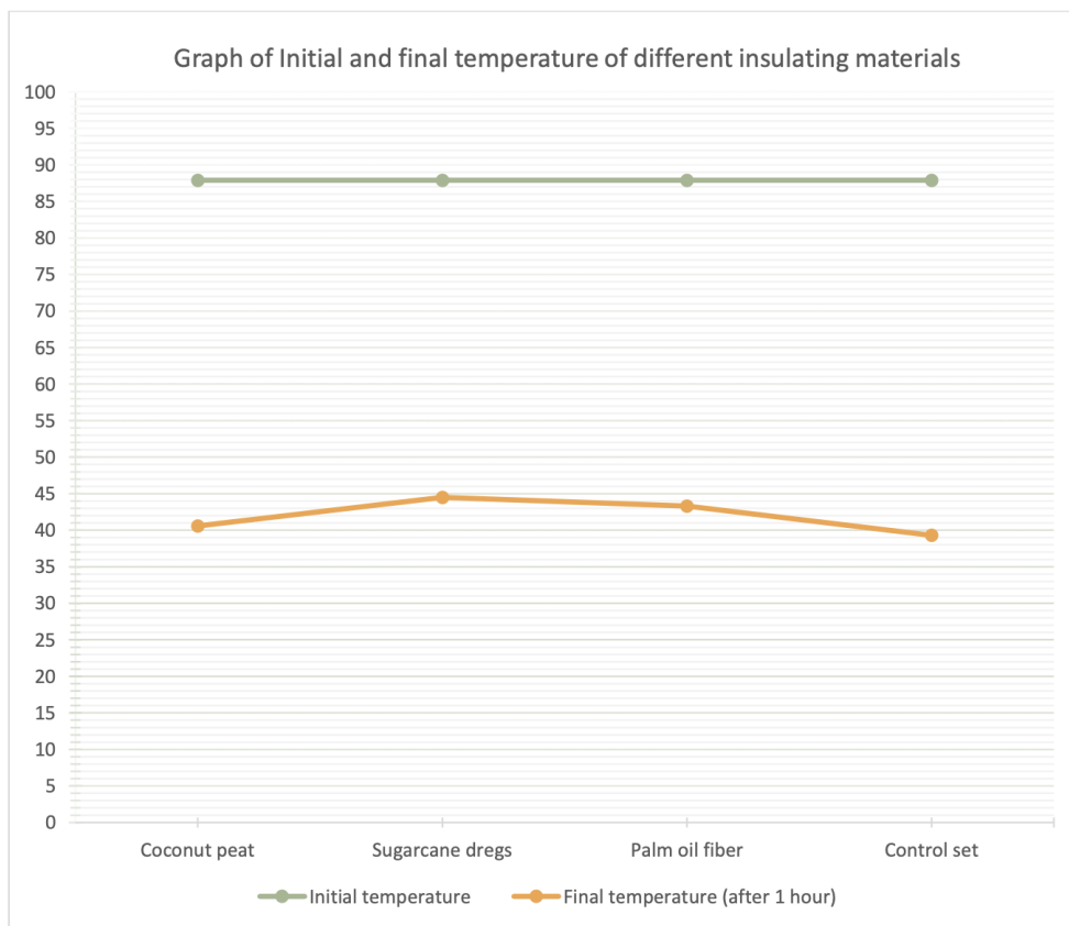
Figure 3 Graph of initial and final temperature of different insulating materials
